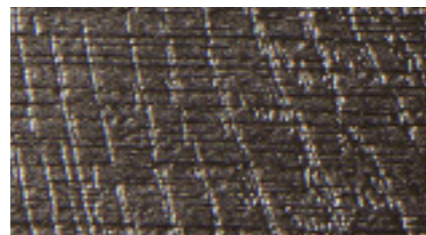
Rough sawn surface
